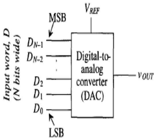
Fig.2: General representation of N-bit DAC
