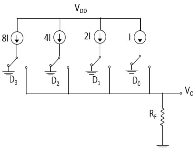
Fig.3: Current Steering DAC with 4 bit binary weight
