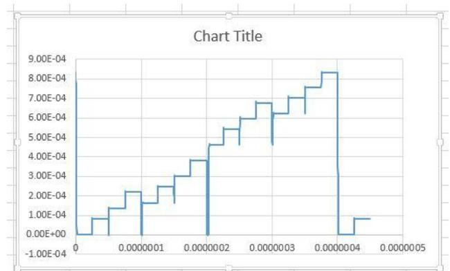
**Fig.7: Output of binary weighted DAC**
