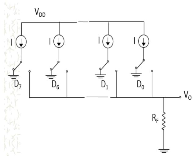
Fig.4: 3-bit current Steering DAC with unary weight
