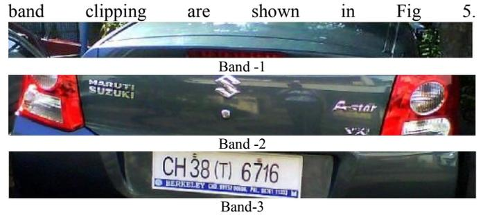
Fig. 5 Bands after vertical band clipping
