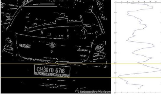
Fig. 3 Vertical projection of edge image
