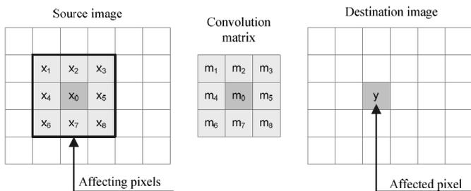
Figure 1 pixel affected by neighbours according to convolution matrix [7]
