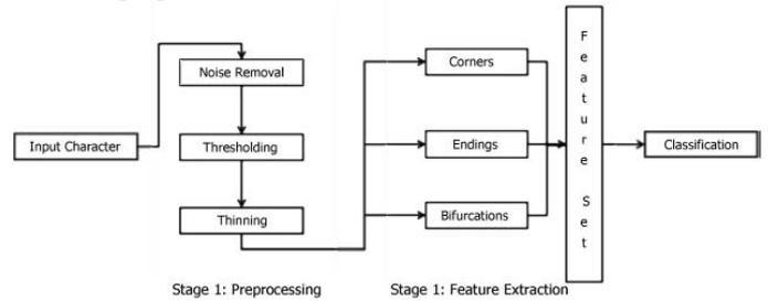
Fig. 11. Block diagram of feature extraction based OCR
