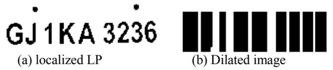
Fig 9 Image dilation on number plate
